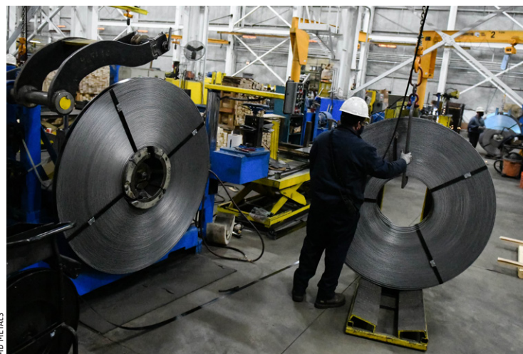
Narrow slitting and edge-conditioning of heavy-gauge steel is a specialty of MD Metals
